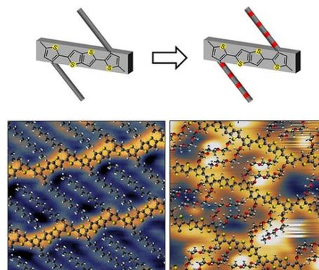
Fig 1: PBTTT & P(G2T-TT) Polymorphs under a Scanning Tunneling Microscope [2]
