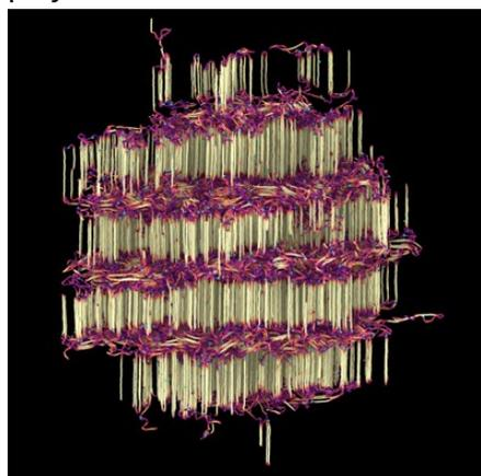
Fig 2: Multilamellar PE crystal grown by the TSP team at ICS using MD [3].
